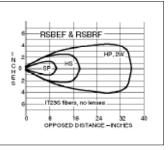
This sensor pair is designed for opposed mode operation using Banner glass fiber optics. Maximum range (HP mode) using L9 lenses is 12 feet. Maximum range using L16F lenses is 50 feet.
