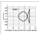
Powerful visible red beam with precise .06" diameter sensing spot. Useful in many high-contrast color registration applications.
