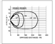
MAXI-BEAM emitters have a visible red "tracer beam". This beam is non-active, and is used as a means of visual alignment during installation. A retroreflector temporarily attached to the receiver lens provides an effective target for the tracer beam during alignment. The narrow beam of the RSBESR/RSBRSR pair is ideal for sensing small parts (effective beam diameter is 0.14 inch).
